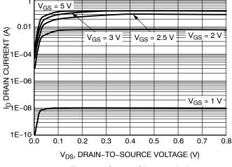
Figure 8. Output Characteristics
