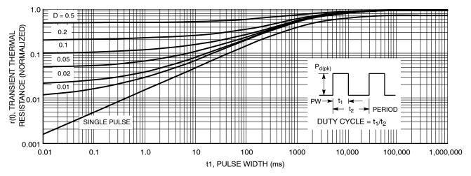
Figure 13. Transient Thermal Response for NUD3124LT1G
