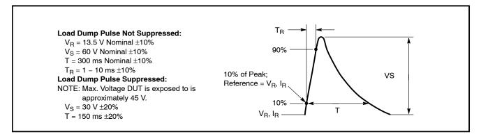
Figure 3. Load Dump Waveform Definition
