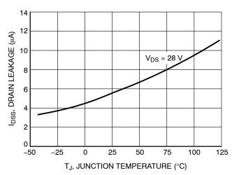
Figure 5. Drain-to-Source Leakage versus Junction Temperature
