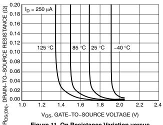
Figure 11. On Resistance Variation versus Gate-to-Source Voltage
