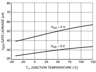
Figure 6. Gate-to-Source Leakage versus Junction Temperature
