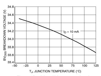
Figure 7. Breakdown Voltage versus Junction Temperature
