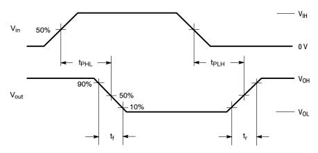
Figure 1. Switching Waveforms
