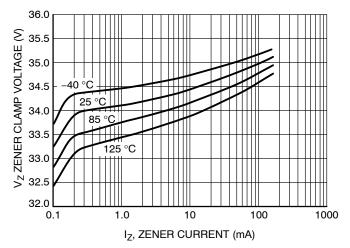
Figure 12. Zener Clamp Voltage versus Zener Current
