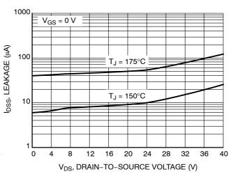
Figure 6. Drain-to-Source Leakage Current vs. Voltage
