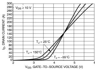
Figure 2. Transfer Characteristics
