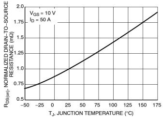
Figure 5. On–Resistance Variation with Temperature
