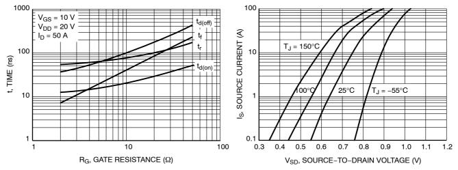
Figure 9. Resistive Switching Time Variation vs. Gate Resistance
