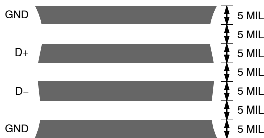
Figure 22. Typical Arrangement of Signal Tracks
