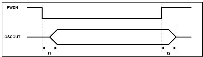
Figure-18. Power Up/Down Timing
