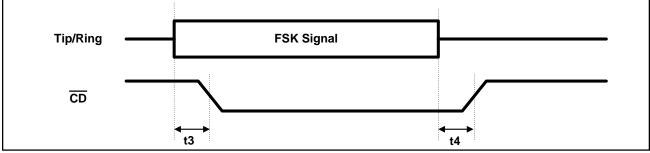
Figure-19. FSK Detection Time
