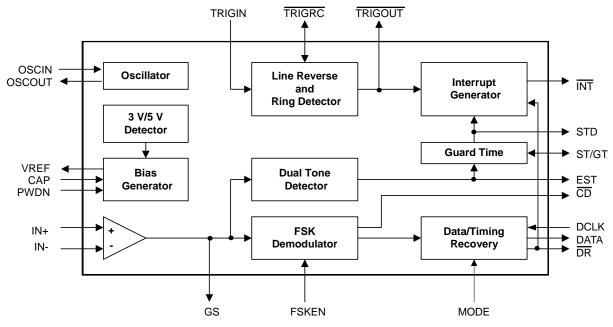
Figure-1. Block Diagram
