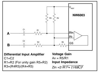
Figure-3. Differential Input Gain Control Circuit
