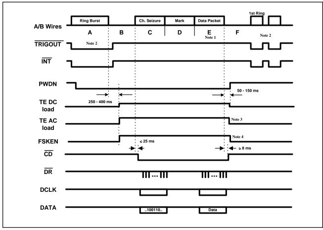
Figure-17. CCA Caller Display Service Timing Diagram
