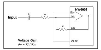
Figure-4. Single-ended Input Gain Control Circuit
