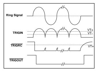
Figure- 5. TRIGIN, TRIGRC and TRIGOUT Operation
