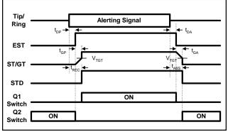
Figure-8. Guard Time Waveform
