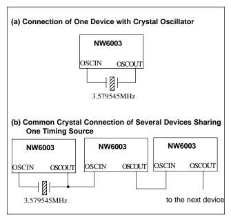
Figure-10. Application of Clock Driven Circuit
