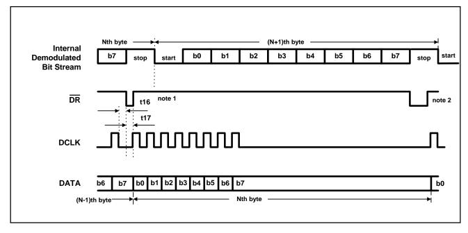
Figure-22. Serial Data Interface Timing in MODE '1'
