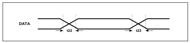
Figure-23. DATA Output Timing in Mode '0'
