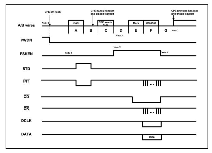
Figure-14. Bellcore Off-hook Data Transmission Timing Diagram
