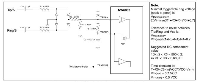
Figure-6. CLIP/CID Call Arrival Detection Circuit
