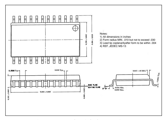
Figure-25. NW6003-XS 24 Pin SOIC Package Diagram
