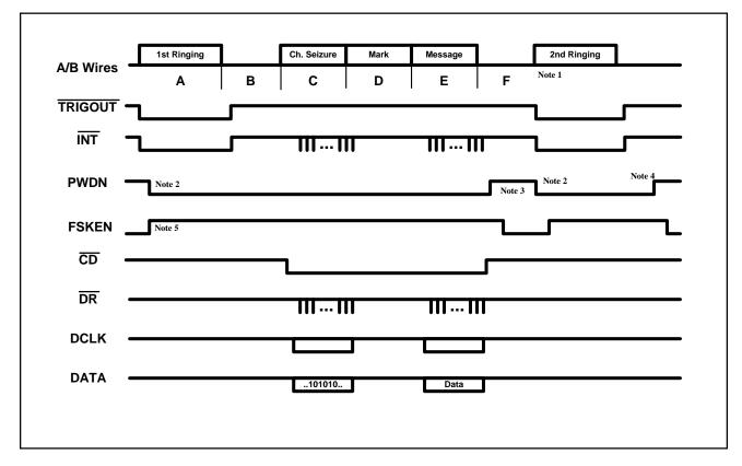
Figure-13. Bellcore On-hook Data Transmission Timing Diagram
