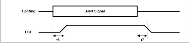
Figure-20. Dual Tone Alert Signal Detection Time
