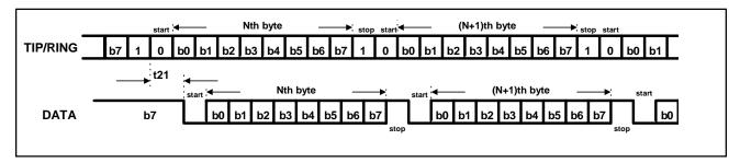
Figure-24. Serial Data Interface Timing in MODE '0'
