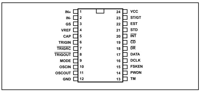
Figure-2. Pin Assignment
