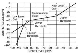
Figure 6. Independent Channel I/O Curve Flexibility
