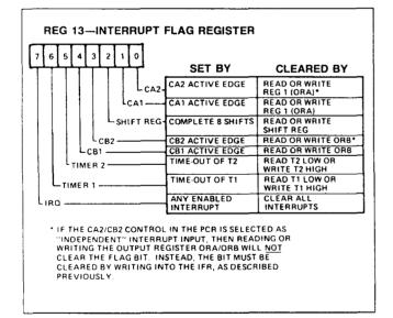
status of the IRQ output. This bit corresponds to the logic function:  $\overline{IRQ} = IFR6 \times IER6 + IFR5 \times IER5 + IFR4 \times IER4 + IFR3 \times IER3 + IFR2 \times IER2 + IFR1 \times IER1 + IFR0 \times IER0.$
