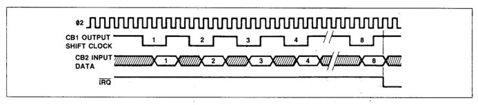
Figure 24. SR Mode 3 — Shift In Under CB1 Control
