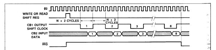
Figure 22. SR Mode 1 — Shift In Under T2 Control
