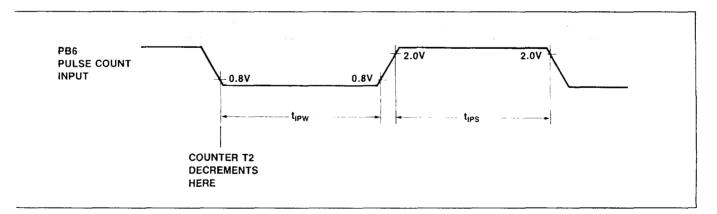
Figure 31i. Pulse Count Input Timing
