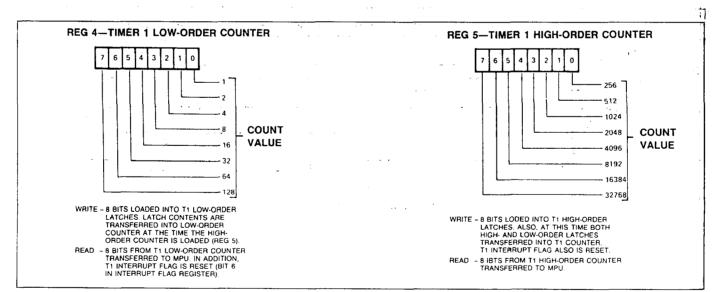
Figure 13. Timer 1 (T1) Counter Registers
