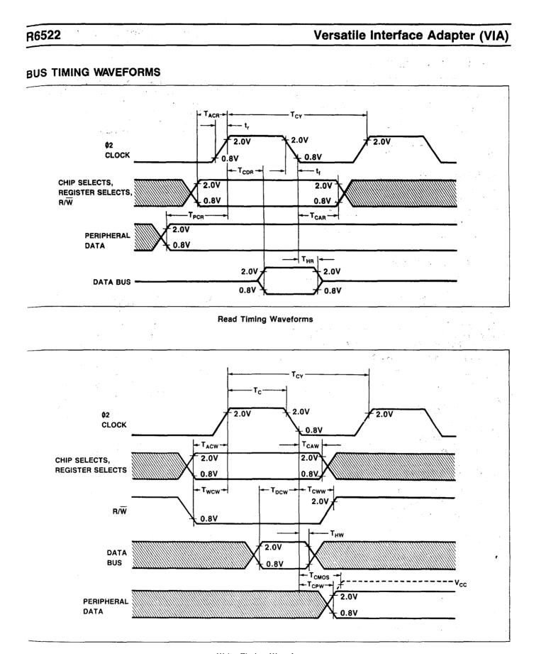
Write Timing Waveforms
