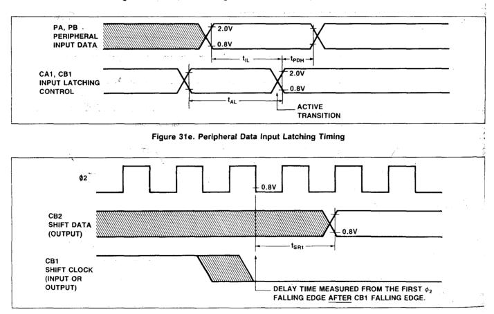
Figure 31f. Timing for Shift Out with Internal or External Shift Clocking
