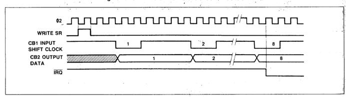
Figure 28. SR Mode 7 --- Shift Out Under CB1 Control
