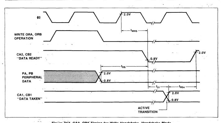
Figure 31d. CA2, CB2 Timing for Write Handshake, Handshake Mode
