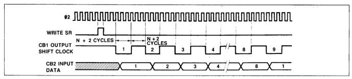
Figure 25. SR Mode 4 — Shift Our Under T2 Control (Free-Run)
