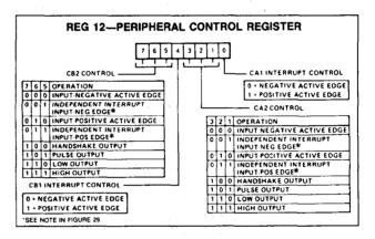
Figure 11. Peripheral Control Register (PCR)
