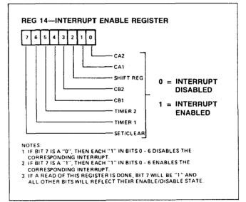
Figure 30. Interrupt Enable Register (IER)
