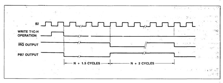
Figure 16. Timer 1 Free-Run Mode Timing
