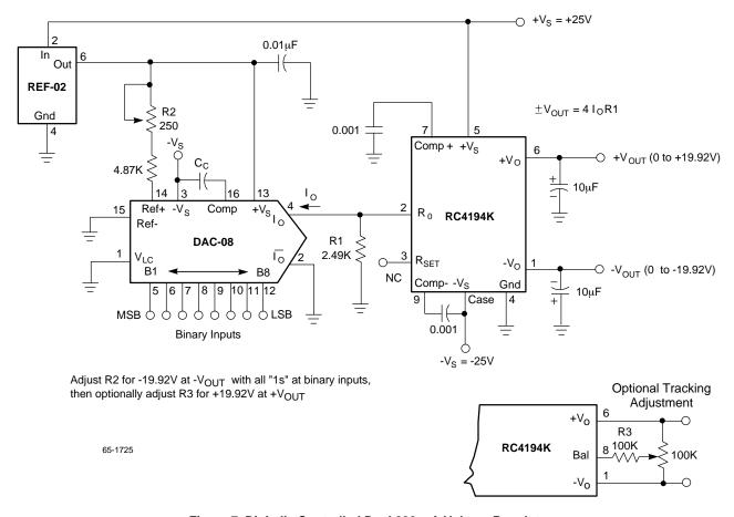
Figure 7. Digitally Controlled Dual 200 mA Voltage Regulator
