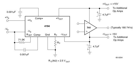
Figure 6. Balanced Output Voltage — Op Amp Application
