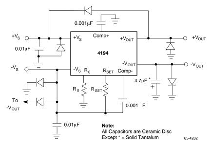
Figure 10. RC4194 Regulator Showing All Protective Diodes
