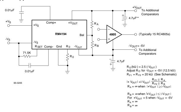
Figure 4. Unbalanced Output Voltage — Comparator Application
