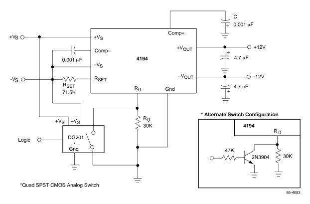
Figure 8. ±12V Switchable Power Supply
