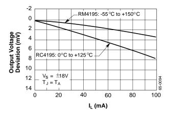
Figure 1. Output Load Regulation
