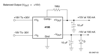
Figure 10. Typical Application Circuit
