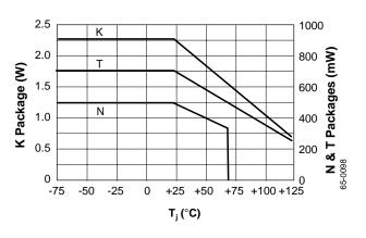
Figure 4. Power Dissipation
