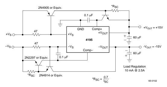
Figure 9. High Output Current
