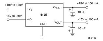
Figure 7. Balanced Output (Vout =  $\pm 15V$ )
