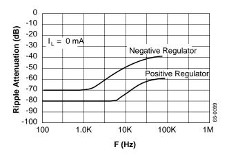
Figure 6. Ripple Rejection
