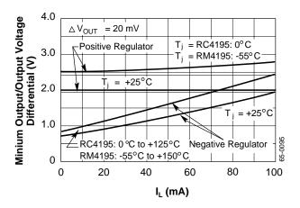
Figure 3. Regulator Dropout Voltage
