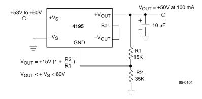
Figure 8. Positive Single Supply (+15V < Vout < +50V)
