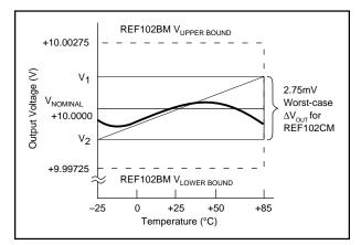
FIGURE 1. REF102CM Output Voltage Drift.
