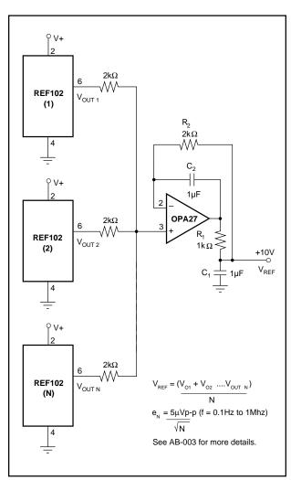
FIGURE 14. Precision Voltage Reference with Extremely Low Noise.
