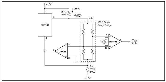
FIGURE 8. Strain Gauge Conditioner for  $350\Omega$  Bridge.
