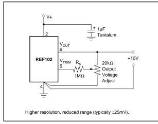
FIGURE 4. REF102 Optional Output Voltage Fine Adjust.
