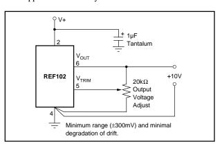
FIGURE 3. REF102 Optional Output Voltage Adjust.
