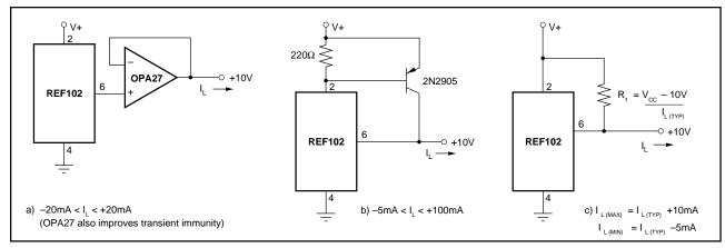
FIGURE 7. +10V Reference With Output Current Boosted to: a) ±20mA, b) +100mA, and c) I<sub>L (TYP)</sub> +10mA, -5A.
