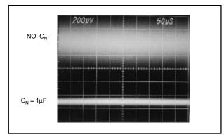
FIGURE 5. Effect of 1µF Noise Reduction Capacitor on Broadband Noise ( $f_{-3dB} = 1MHz$ ).
