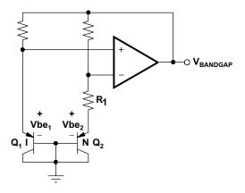
Figure 3. Simplified Schematic of Bandgap Reference
