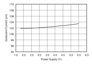
Figure 5. Supply Current vs Supply Voltage
