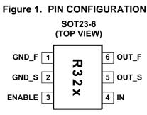
A. The location of pin 1 on the REF32xx is determined by orienting the package marking as shown.
