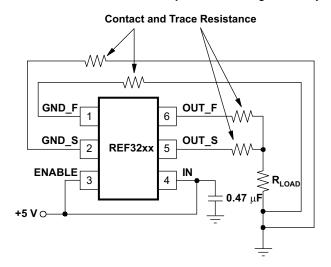
Figure 7. Accurate Load Regulation of REF32xx
