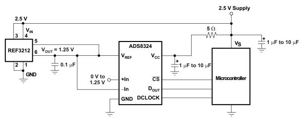
Figure 10. Basic Data Acquisition System 2
