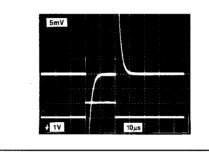
FIGURE 2C: Pulse Response with Output Decoupling
