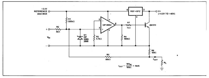
The current transmitter of Figure 10 provides an output of 4mA to 20mA that is linearly proportional to the input voltage. Linearity of the transmitter exceeds 0.004% and line rejection is below measurement limits.
