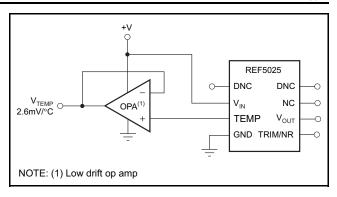
Figure 28. Buffering the TEMP Pin Output
