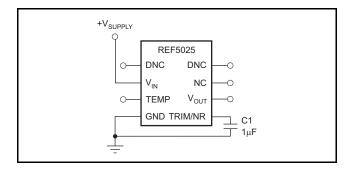
Figure 27. Noise Reduction Using TRIM/NR Pin
