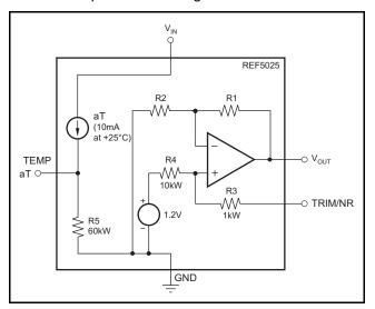
Figure 24. REF5025 Simplified Block Diagram
