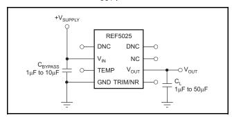
Figure 25. Basic Connections
