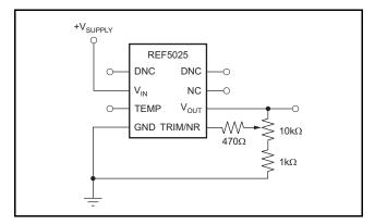
Figure 26. V<sub>OUT</sub> Adjustment Using TRIM/NR Pin
