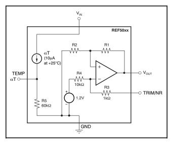
Figure 28. REF50xx Simplified Block Diagram
