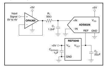
Figure 34. Basic Data Acquisition System
