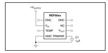
Figure 31. Noise Reduction Using TRIM/NR Pin
