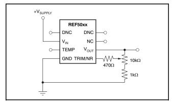
Figure 30. V<sub>OUT</sub> Adjustment Using TRIM/NR Pin
