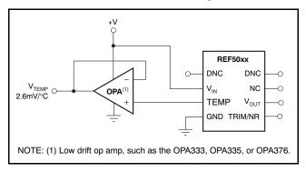
Figure 32. Buffering the TEMP Pin Output
