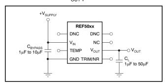
Figure 29. Basic Connections
