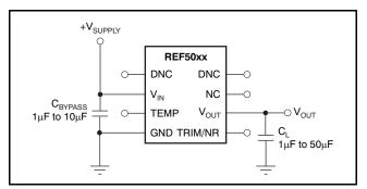
Figure 23. Basic Connections
