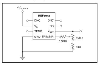
Figure 24. V<sub>OUT</sub> Adjustment Using the TRIM/NR Pin
