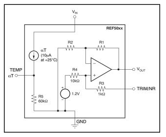
Figure 22. REF50xx Simplified Block Diagram
