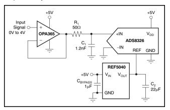
Figure 28. Basic Data Acquisition System
