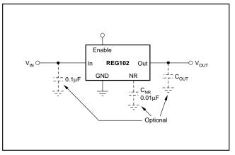
FIGURE 1. Fixed Voltage Nominal Circuit for the REG102.
