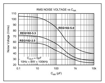
FIGURE 5. Output Noise versus Noise Reduction Capacitor.
