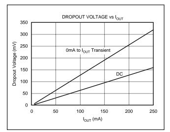
FIGURE 6. Transient and DC Dropout.
