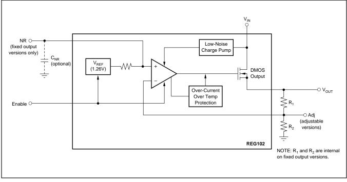
FIGURE 4. Block Diagram.
