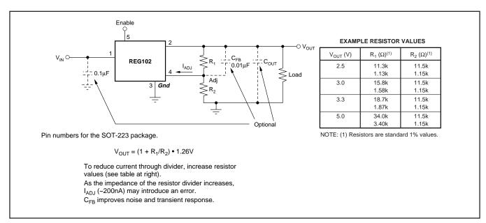
FIGURE 2. Adjustable Voltage Circuit for the REG102A.
