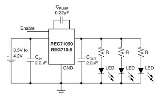
Figure 14. Circuit for Driving LEDs
