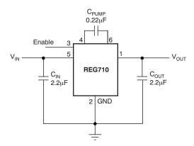
Figure 10. Typical Operating Circuit
