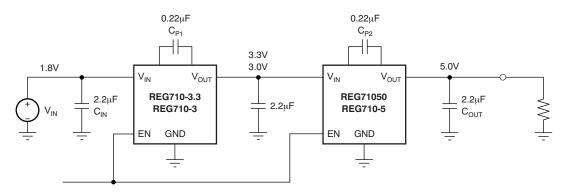
Figure 12. Circuit for Step-Up Operation From 1.8 V to 5 V With 10-mA Output Current
