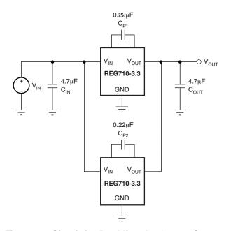
Figure 13. Circuit for Doubling the Output Current
