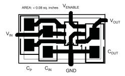
Figure 11. Suggested PCB Design for Minimum Ripple
