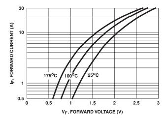
FIGURE 1. FORWARD CURRENT vs FORWARD VOLTAGE
