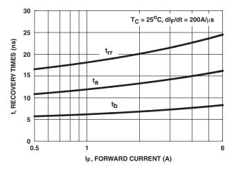
FIGURE 3.  $t_{\rm rr}, t_{\rm a}$  AND  $t_{\rm b}$  CURVES vs FORWARD CURRENT
