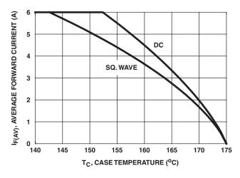
FIGURE 6. CURRENT DERATING CURVE
