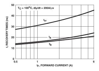
FIGURE 4. t<sub>rr</sub>, t<sub>a</sub> AND t<sub>b</sub> CURVES vs FORWARD CURRENT
