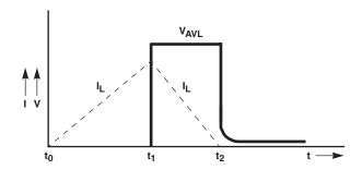
FIGURE 11. AVALANCHE CURRENT AND VOLTAGE WAVEFORMS
