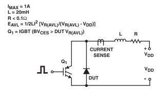
FIGURE 10. AVALANCHE ENERGY TEST CIRCUIT
