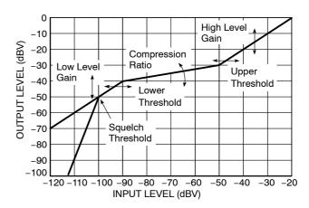
Figure 5. Independent Channel I/O Curve Flexibility
