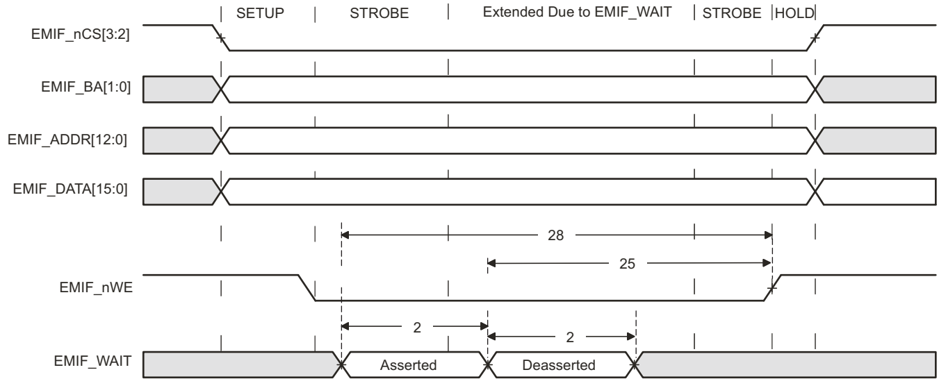
Figure 4-15. EMIFnWAIT Write Timing Requirements
