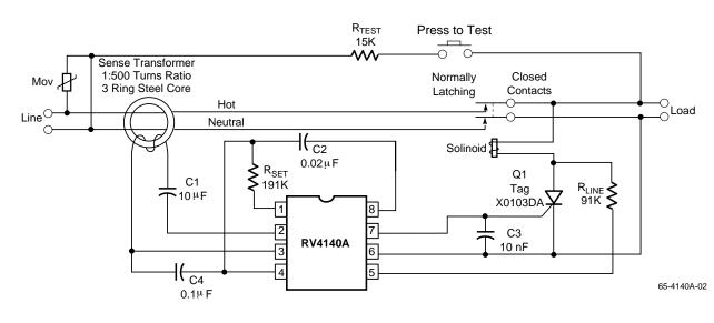
Figure 1. Appliance Leakage Detector Circuit Application
