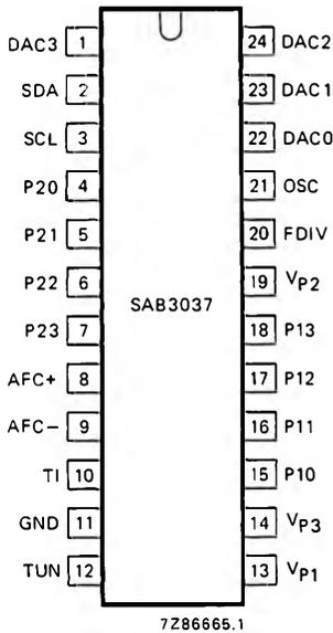
Fig. 2 Pinning diagram.
