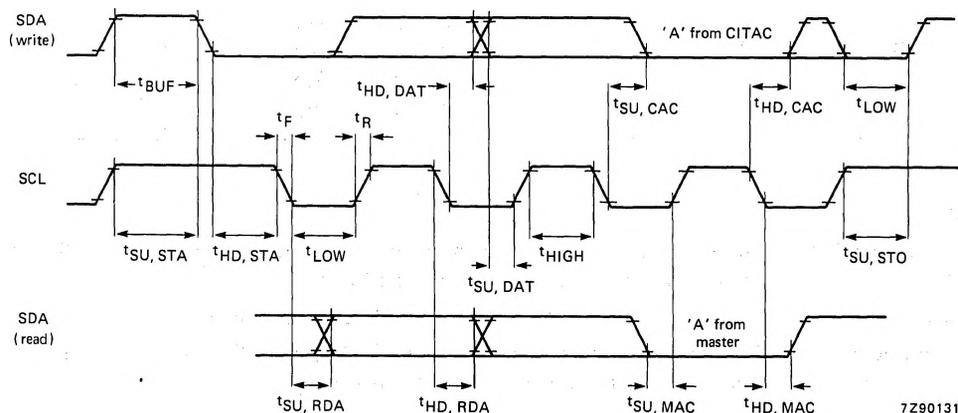
Fig. 8 I<sup>2</sup>C bus timing SAB3037.
