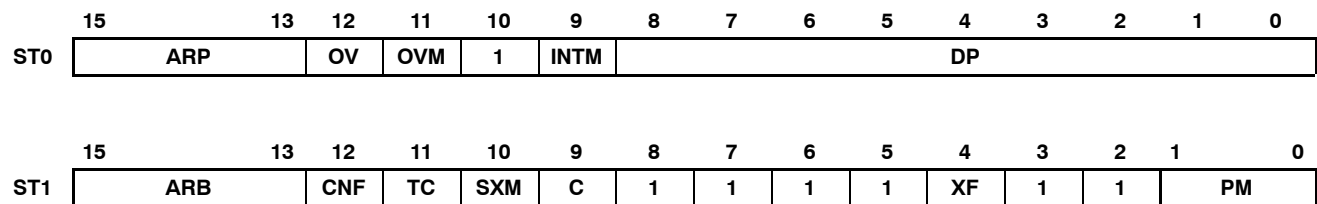
Figure 10. Status and Control Register Organization
