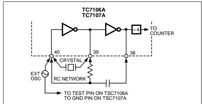
**Figure 6. Clock Circuits**
