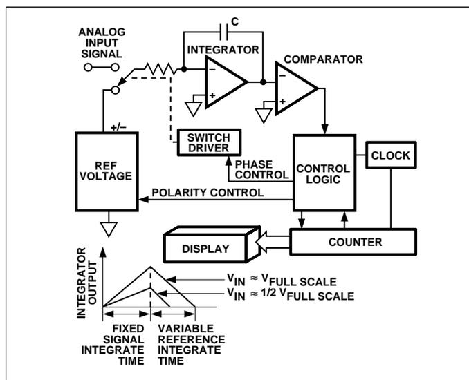
Figure 2A. Basic Dual Slope Converter
