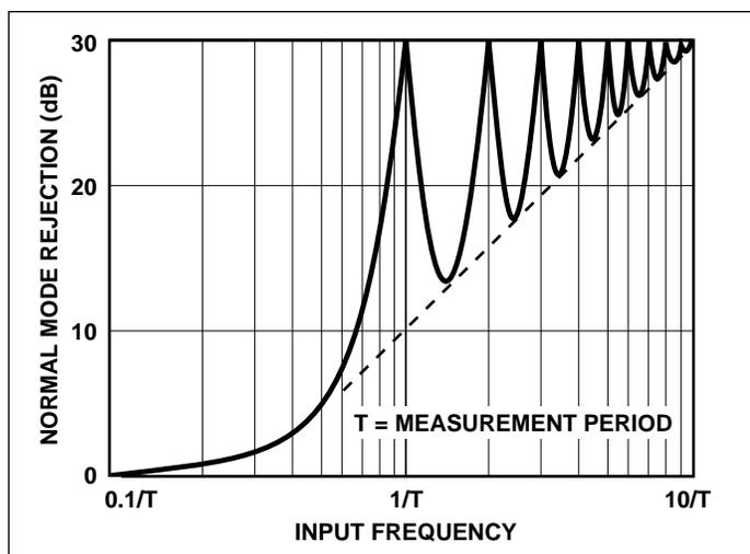
Figure 2B. Normal-Mode Rejection of Dual Slope Converter
