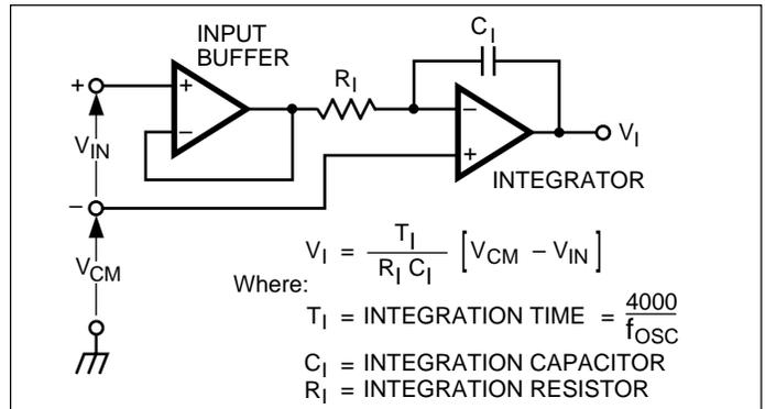
Figure 9. Common-Mode Voltage Reduces Available Integrator Swing. ( $V_{COM} \neq V_{IN}$ )
