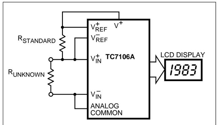
Figure 17. Low Parts Count Ratiometric Resistance Measurement
