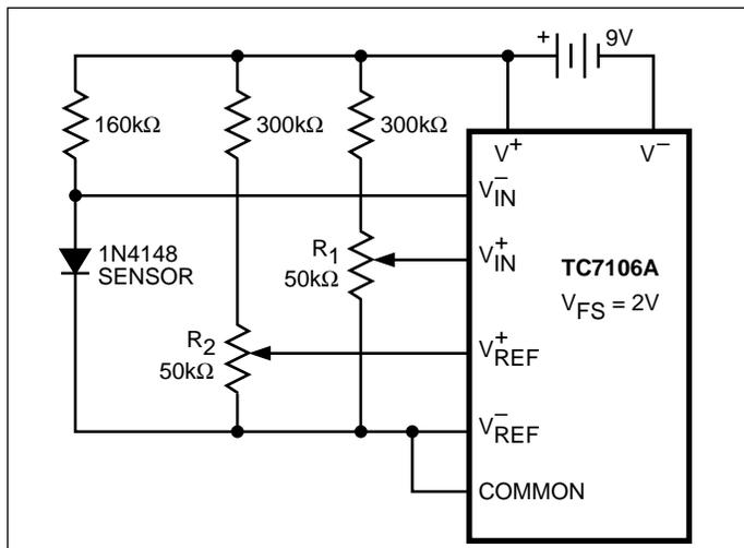
Figure 19. Temperature Sensor
