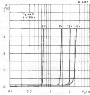
Fig. 8 - Distortion vs. output power
