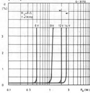
Fig. 11 - Distortion vs. output power
