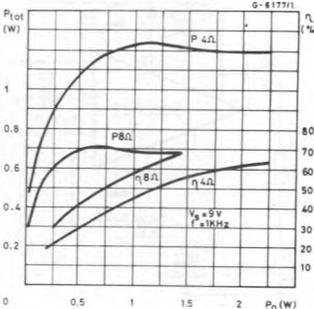
Fig. 20 - Total power dissipation vs. output power
