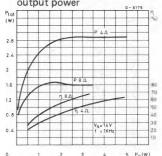
Fig. 18 - Total power dissipation vs. output power
