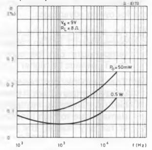
Fig. 15 - Distortion vs. frequency
