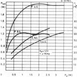
Fig. 19 - Total power dissipation vs. output power
