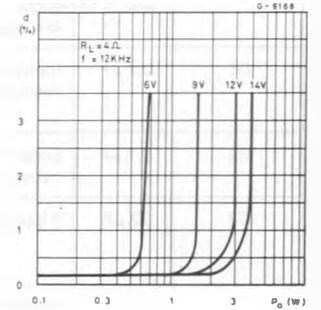
Fig. 9 - Distortion vs. output power
