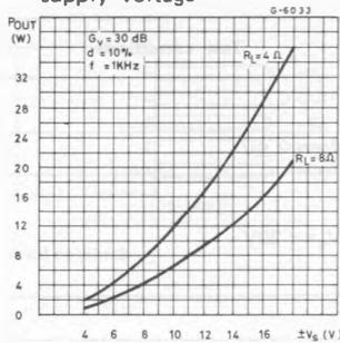
Fig. 3 - Output power vs. supply voltage
