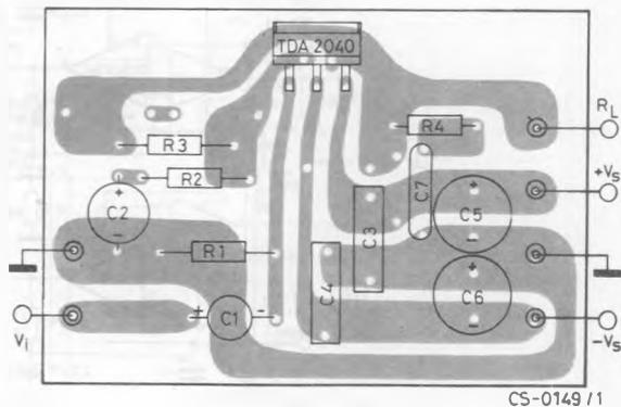
Fig. 12 - Amplifier with single supply (\*)
