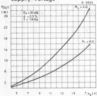
Fig. 2 - Output power vs. supply voltage
