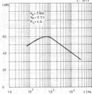
Fig. 6 - Supply voltage rejection vs. voltage gain
