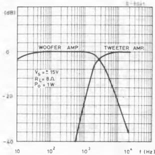
Fig. 19 - Power distribution vs. frequency
