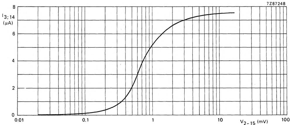
Fig. 2 Typical Q-factor killer current (pins 3 and 14) as a function of the peak-to-peak input voltage ( $V_{2-15}$ );  $I_{3, 14}$  is measured to ground,  $V_{2-15(p-p)}$  is a symmetrical square wave. Measured in Fig. 4;  $V_P = 5\text{ V}$ .
