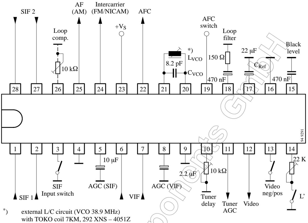
Figure 3. Test circuit
