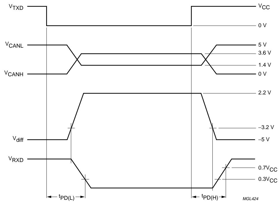
$$V_{\text{diff}} = V_{\text{CANH}} - V_{\text{CANL}}$$
