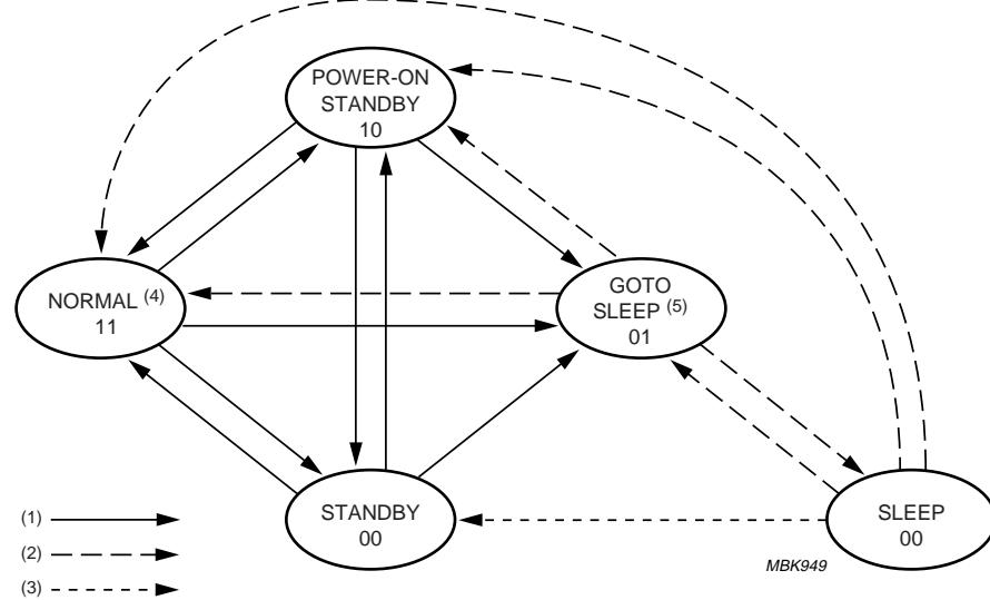
Mode 10 stands for: Pin  $\overline{STB}$  = HIGH and pin EN = LOW.
