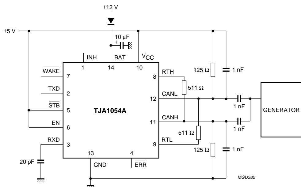
The waveforms of the applied transients on pins CANH and CANL will be in accordance with "ISO 7637 part 1": test pulses 1, 2, 3a and 3b.
