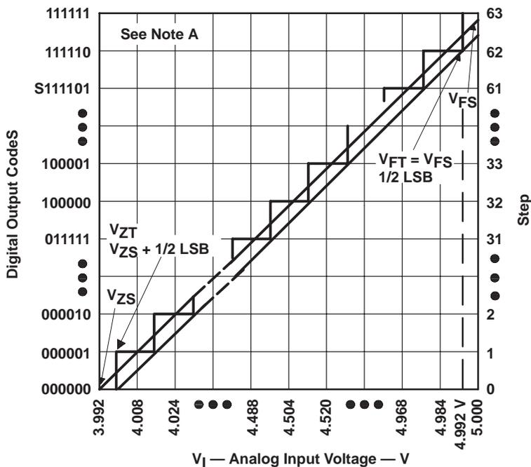
NOTE A: This curve is based on the assumption that  $V_{refB}$  and  $V_{refT}$  have been adjusted so that the voltage at the transition from digital 0 to 1 ( $V_{ZT}$ ) is 4.000 V and the transition to full scale ( $V_{FT}$ ) is 4.992 V. 1 LSB = 16 mV.
