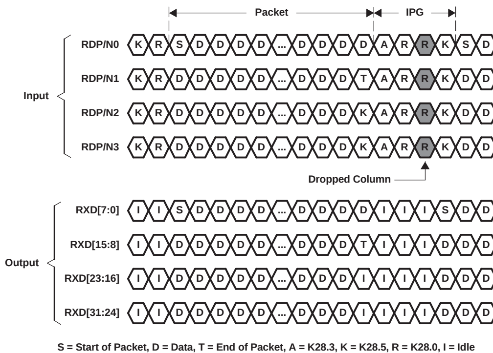
Figure 17. Clock Tolerance Compensation: Drop
