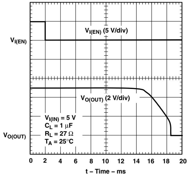
Figure 5. Turnoff Delay and Fall Time
