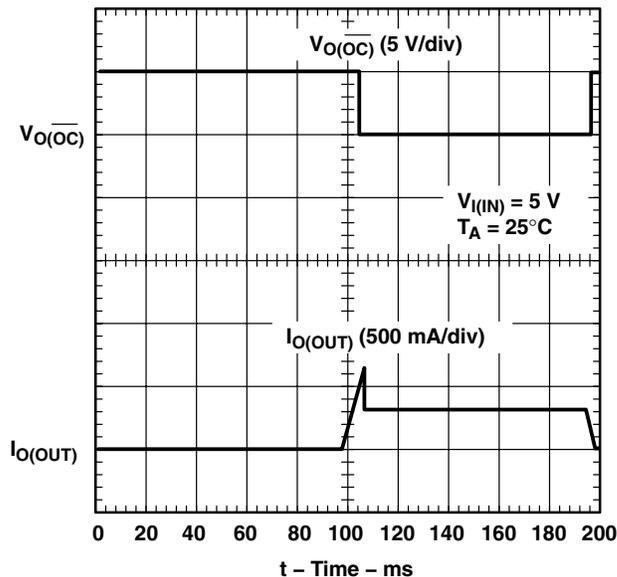
Figure 7. TPS2030, Ramped Load on Enabled Device
