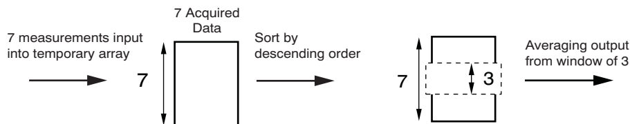
Figure 28. MAV Filter Operation (Patent Pending)
