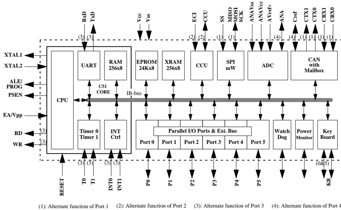
Figure 1. TSC8051A11 block diagram
