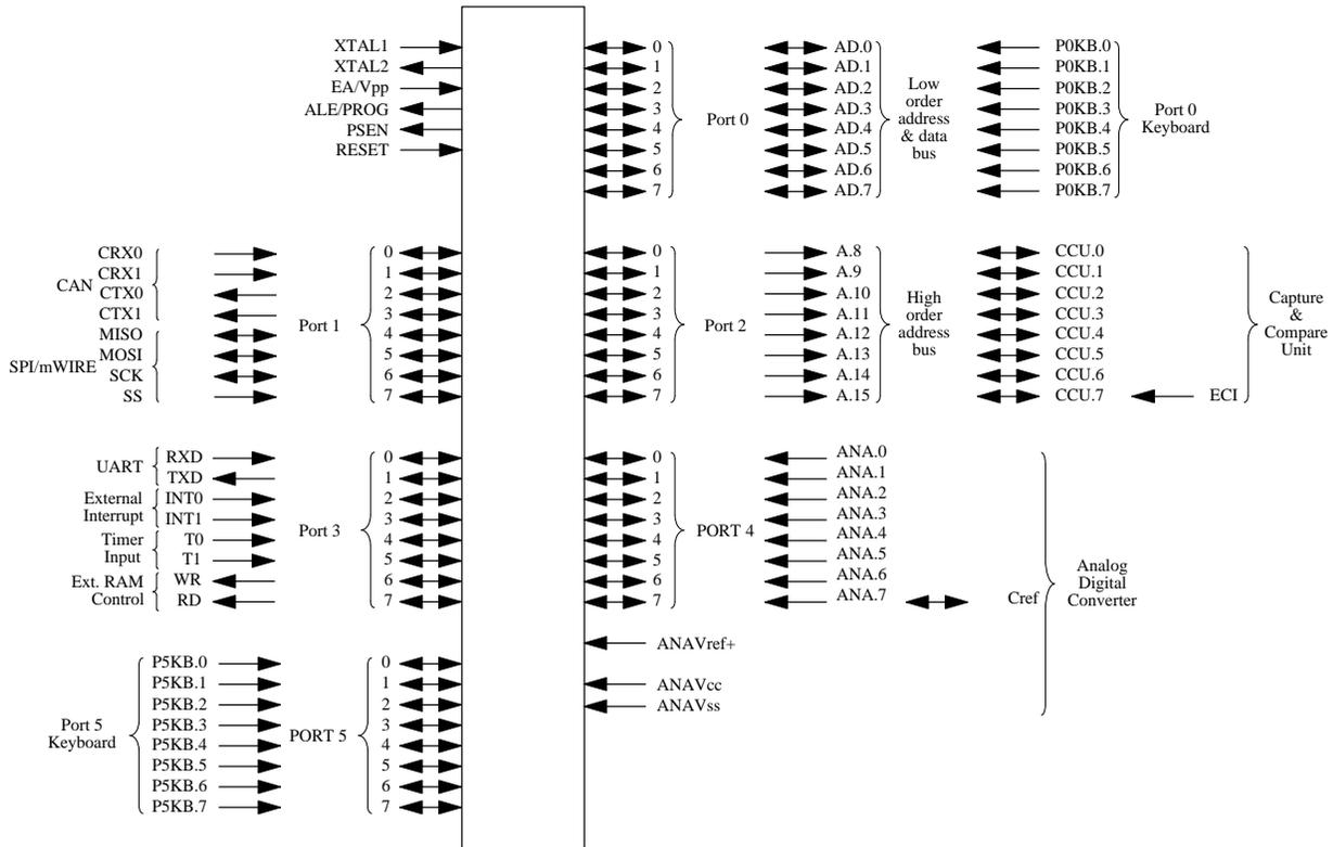
**Figure 2. TSC8051A11 pin functions**
