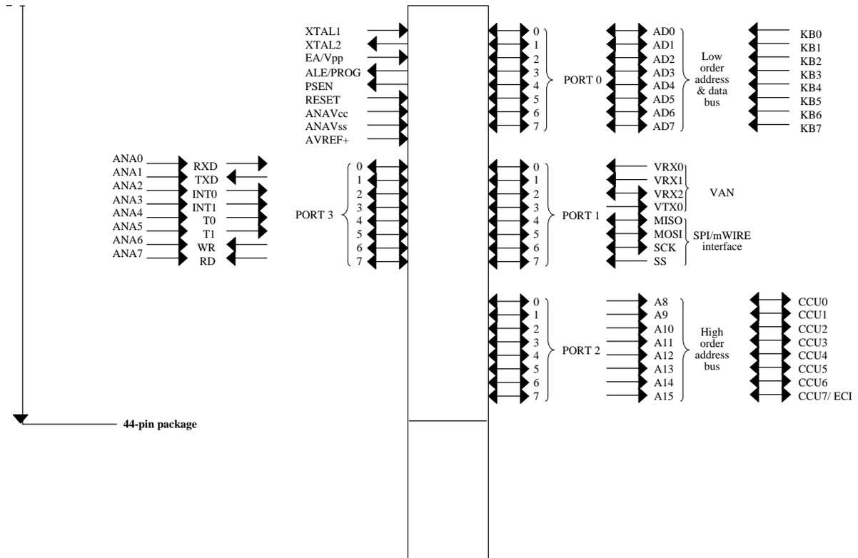
**Figure 2. TSC8051A30 pin functions**
