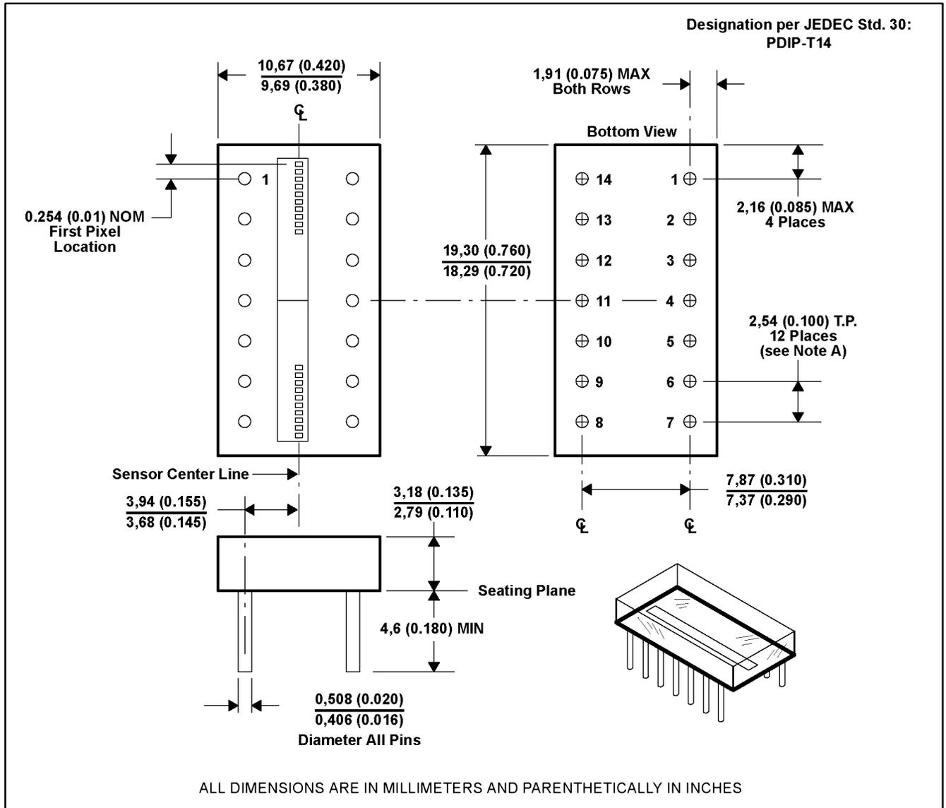
NOTE A: The true-position spacing is 2,54 mm (0.100 inch) between lead centerlines. Each pin centerline is located within 0,25 mm (0.010 inch) of its true longitudinal positions.
