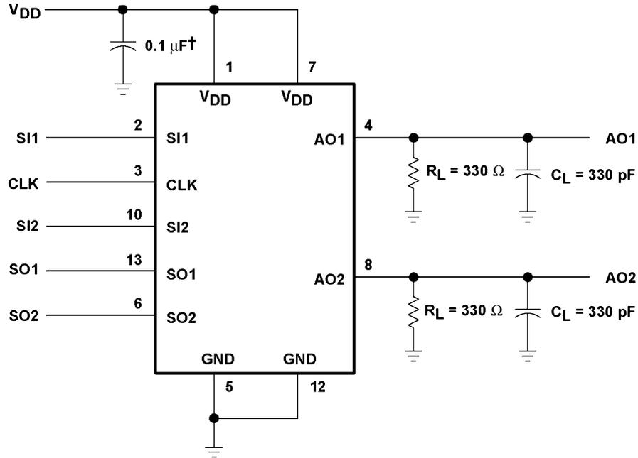
† Supply bypass capacitor with short leads should be placed as close to the device as possible.
