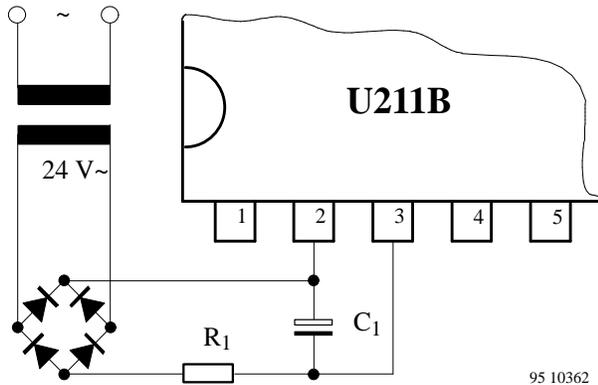
Figure 3. Supply voltage for high current requirements
