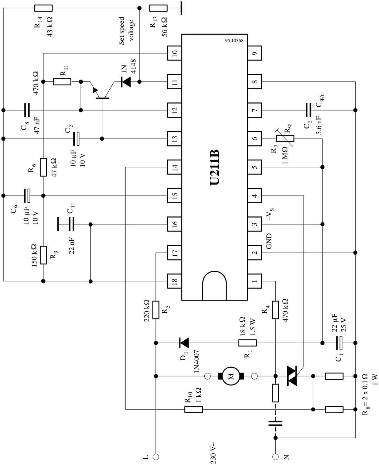
Figure 27. Automatic retriggering, soft-start, reswitching at  $\alpha_{max}$
