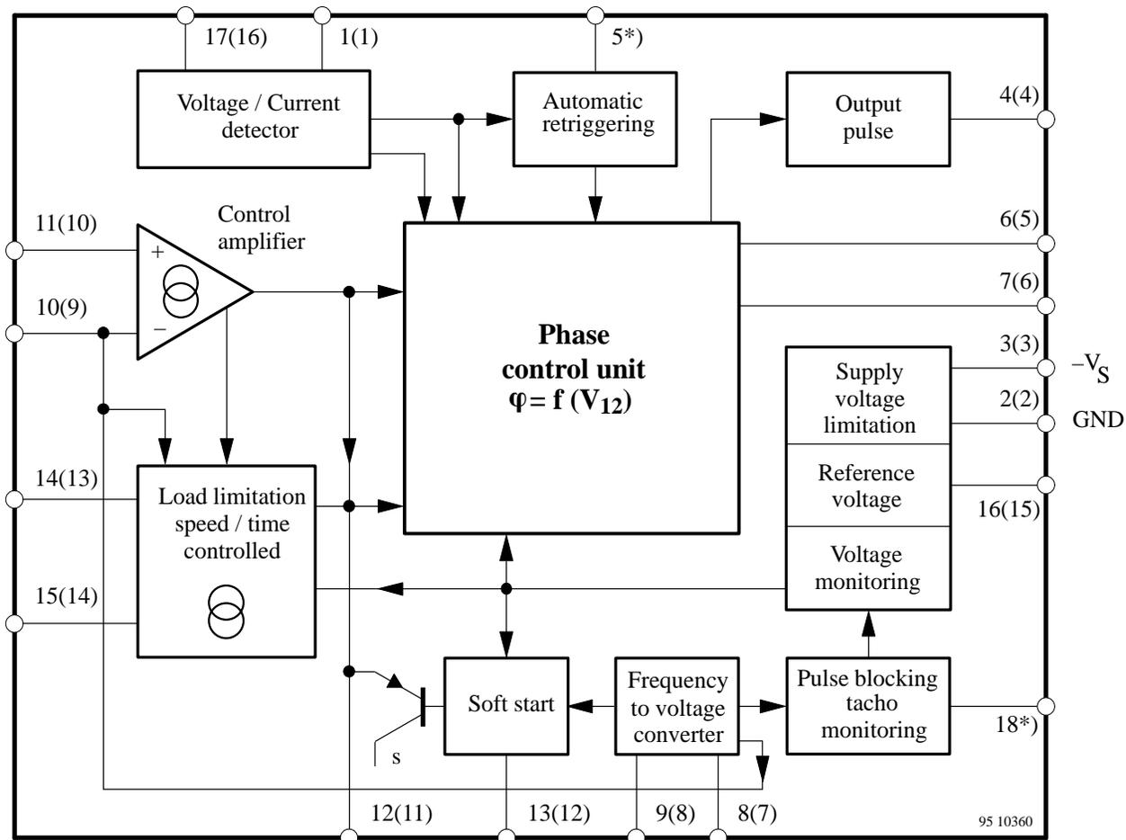
Figure 1. Block diagram ( ) SO 16 \* Pins 5 and 18 connected internally
