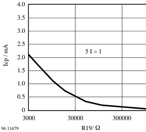
Figure 3. Charge pump characteristics
