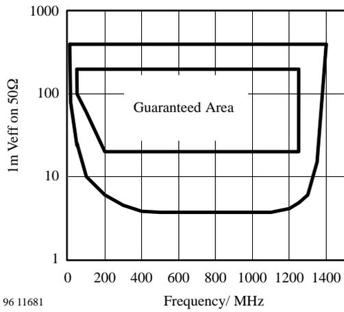
Figure 4. Input sensitivity of PLL1
