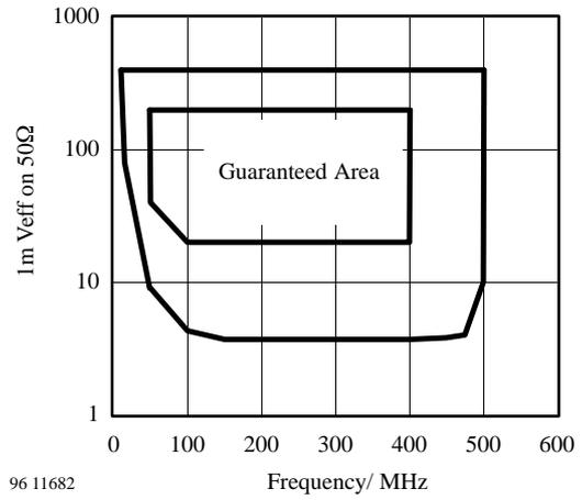
Figure 5. Input sensitivity of PLL2
