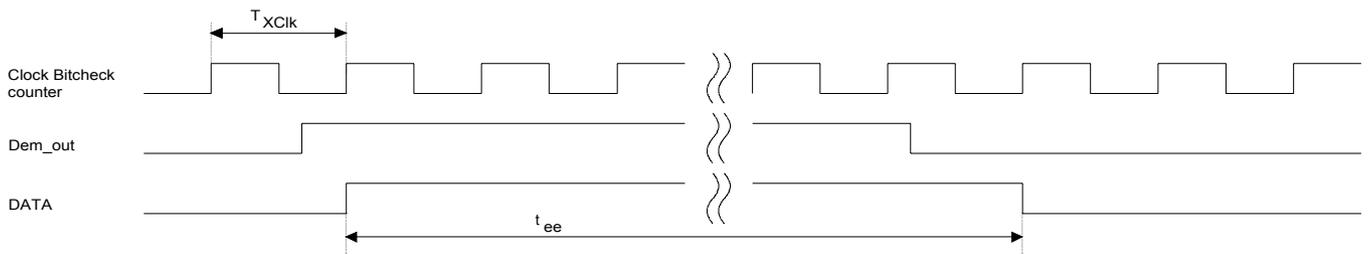
**Figure 15.** Debouncing of the Demodulator Output
