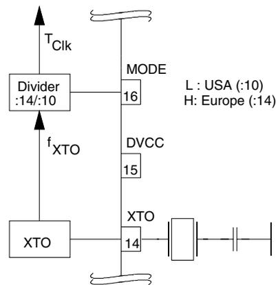
Pin MODE can now be set in accordance with the desired clock cycle  $T_{Clk}$ .  $T_{Clk}$  controls the following application-relevant parameters:
