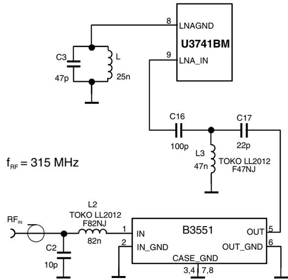
Figure 4. Input Matching Network without SAW Filter
