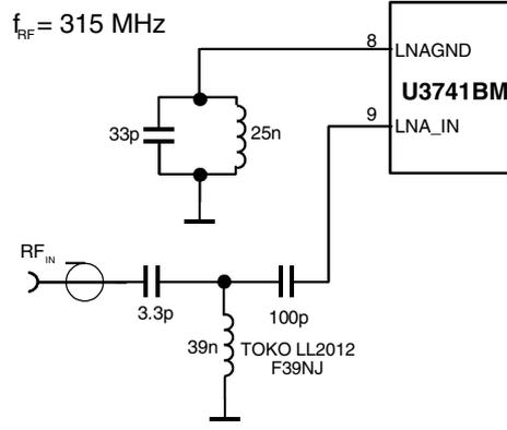
Please note that for all coupling conditions (see Figure 3 and Figure 4), the bond wire inductivity of the LNA ground is compensated. C3 forms a series resonance circuit together with the bond wire. L = 25 nH is a feed inductor to establish a DC path. Its value is not critical but must be large enough not to detune the series resonance circuit. For cost reduction, this inductor can be easily printed on the PCB. This configuration improves the sensitivity of the receiver by about 1 dB to 2 dB.
