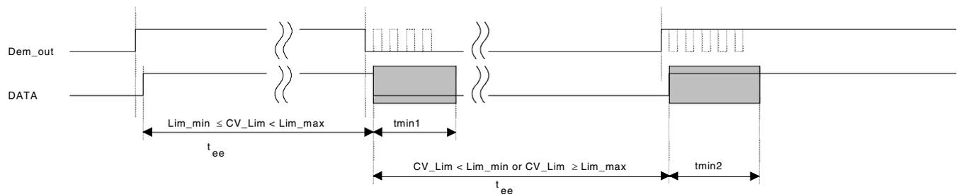
**Figure 16.** Steady L State Limited DATA Output Pattern after Transmission
