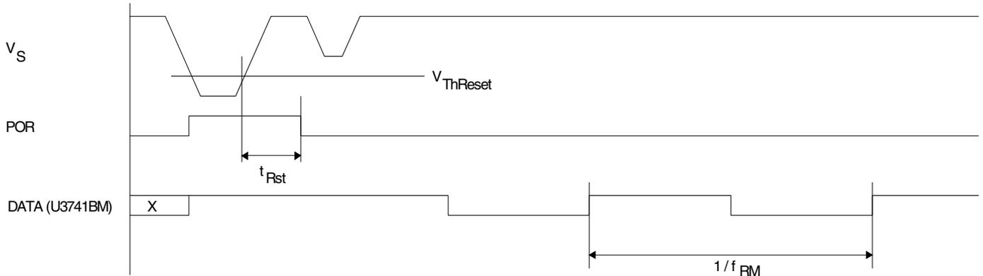
**Figure 20.** Timing of the Register Programming
