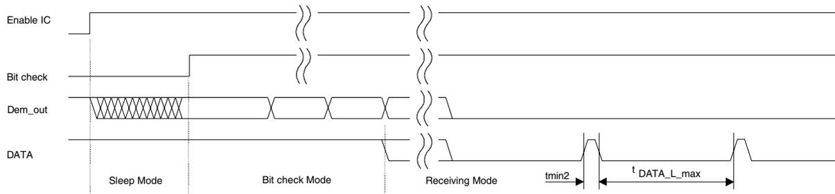
After the end of a data transmission, the receiver remains active and random noise pulses appear at pin DATA. The edge-to-edge time period  $t_{ee}$  of the majority of these noise pulses is equal to or slightly higher than  $T_{DATA\_min}$ .
