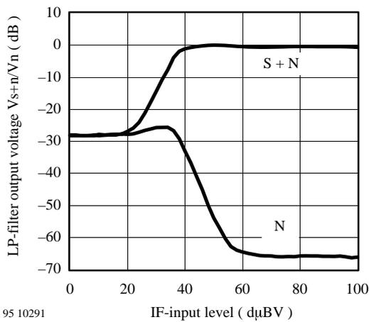
Figure 27. Signal-to-noise ratio FM; deviation 22.5 kHz
