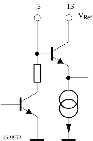
Figure 6. Pin 3 RC<sub>wake</sub>
