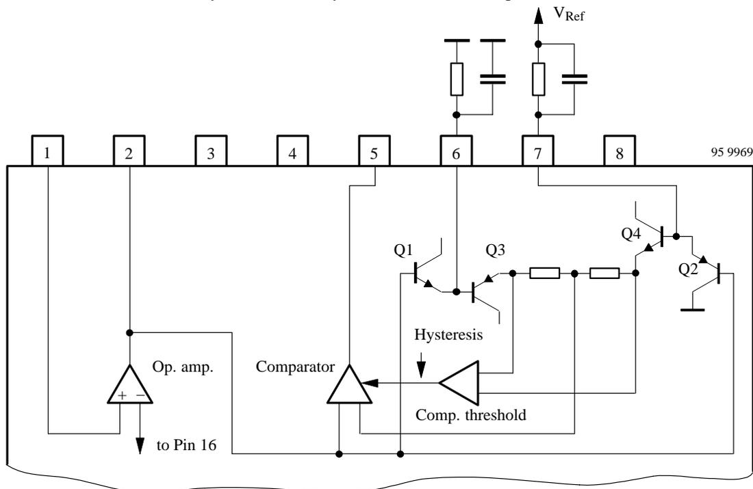
Figure 3. Principle function of the clamping comparator
