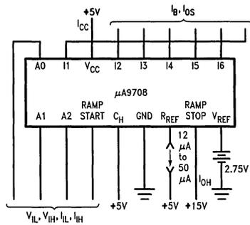
FIGURE 4. Static Measurements
