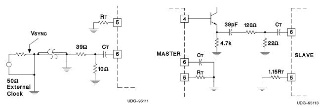
Figure 9. General Oscillator Synchronization
