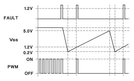
Figure 5. Soft-Start and Fault Waveforms
