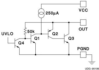
Figure 7. Output V and I During UVLO
