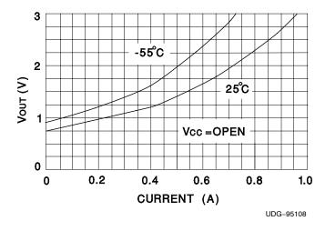
Figure 6. Output Voltage vs Output Current
