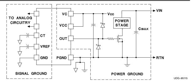
Figure 13. Ground Planes Diagram
