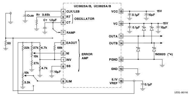
Figure 14. Open Loop Test Circuit Schematic
