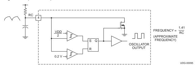
Figure 1. Block Diagram for Oscillator
