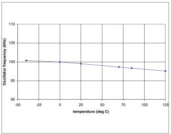
Figure 8. Oscillator frequency vs. temperature.
