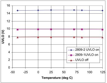
Figure 7. UVLO vs. temperature.
