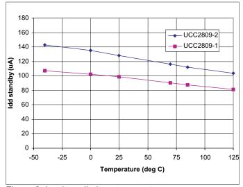
Figure 6. I<sub>DD</sub> (standby) vs. temperature.
