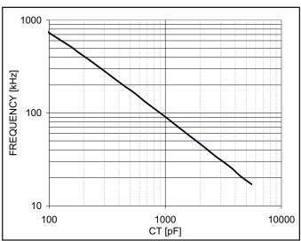
Figure 4. Oscillator frequency vs. C<sub>T</sub> (RT1 = 10k, RT2 = 4.32k)
