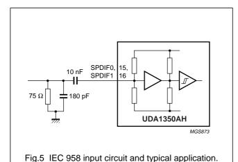
All 24 bits of data for left and right are extracted from the input bitstream as well as several of the IEC 958 key channel-status bits.
