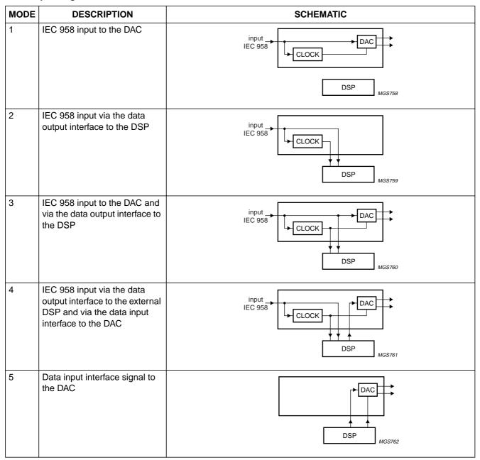
The UDA1350AH is a low cost multi-purpose IEC 958 decoder DAC with a variety of operating modes.
