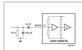
Fig.5 IEC 60958 input circuit and typical application.
