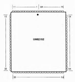
\*A38152 is AUSTEK's cache controller for 25 MHz 386 AT system. Copyright © 1987 AUSTEK Microsystems. All rights reserved.
