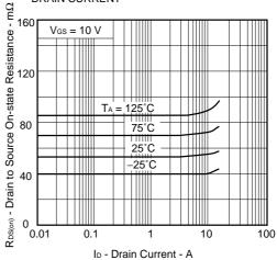
DRAIN TO SOURCE ON-STATE RESISTANCE vs.
