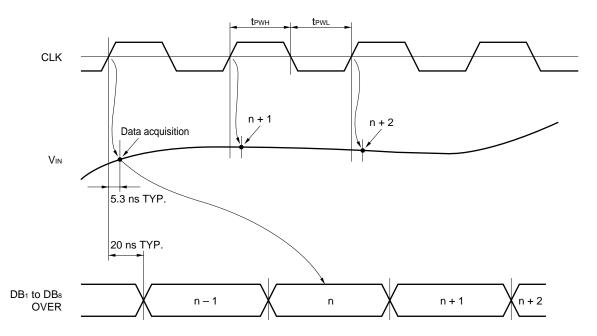
Analog signal is captured at the rising edge, and converted data will be output at the rising edge after 1 clock pulse<sup>Note</sup>.
