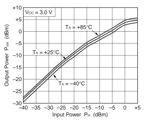
OUTPUT POWER OF EACH TONE, IM<sub>3</sub> vs. INPUT POWER OF EACH TONE
