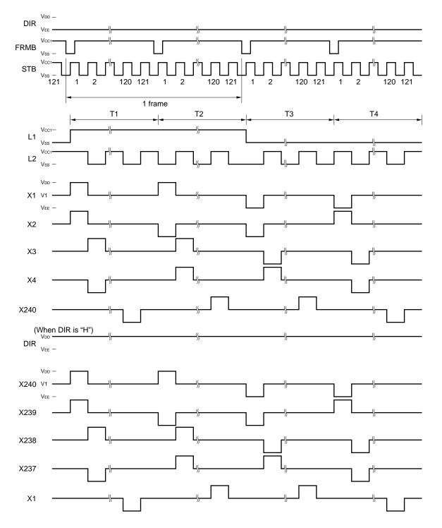
**Remark** While the DOFFB' is "L", the X output remains at the V1 level. Afterward, if it becomes "H", the level of the X output is output timed with the above timing.
