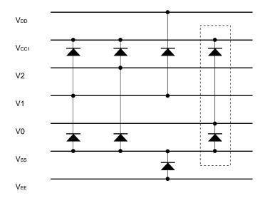
Connect the diodes enclosed in the dotted line when Vo is not 0 V (GND)
